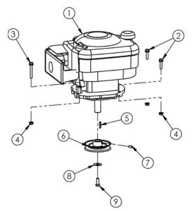
Note: Install pulley collar up and bottom side of pulley flush with end of engine shaft.
