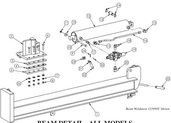
BEAM DETAIL - ALL MODELS NOT ALL PARTS ARE ON ALL MODELS
